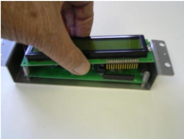
Remove hex spacers and second circuit board then replace spacers in metal pan.
