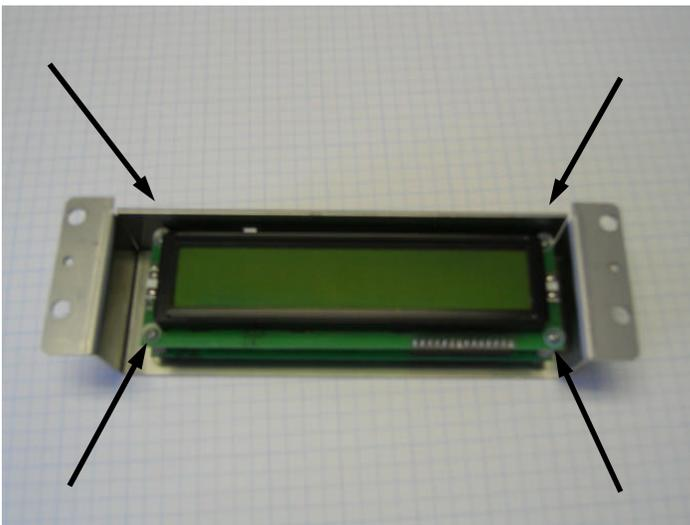
Carefully lift and separate two circuit boards.
