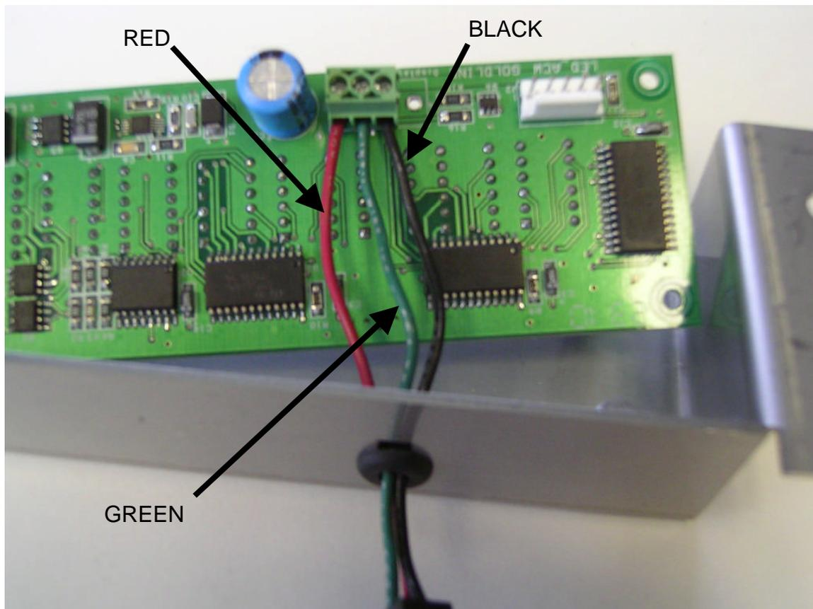
Turn board over and install on metal spacers as shown.
